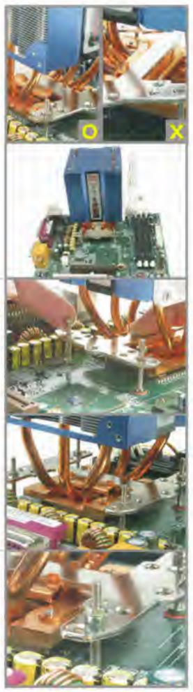
1 7 Tighten additional nut to each screws to ensure proper installation.
